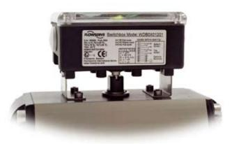
W series switchbox is designed to be directly and easily mounted onto actuators having connections according to Namur VDI/VDE 3845, in order to reduce switchbox/actuator overall dimensions. Picture shows W series with low profile mounting kit KL01. A. WDB01 B. WDB02 C. WDB03
